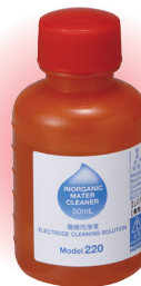
Cleaning Solution 220 (Part no. 3014028653) - contains 10% thiourea and 1% hydrochloric acid (HCl) for removing stubborn deposits on sensor surface
