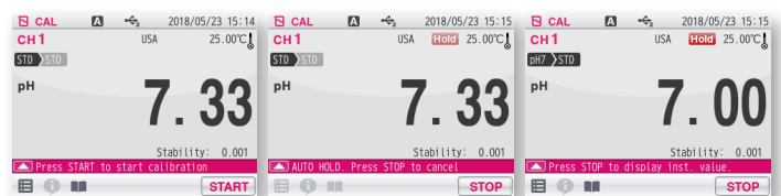
Figure 2: Screenshots of F-74 meter before, during, and after calibration with pH 7 buffer at 25°C
