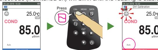
4. Press ENT button to confirm the conductivity reading. To abort calibration, press MEAS button.
