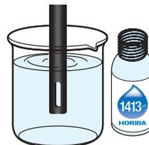
3. Press CAL button on the meter to switch to calibration mode.
