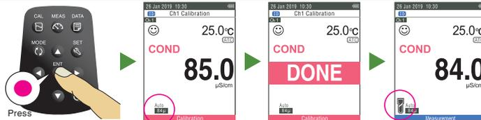
5. Repeat step nos. 1 to 4 to perform calibration with the next standard solution(s).
