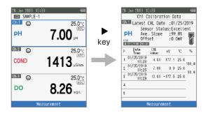
In the focused ID of the measurement mode, the sensor condition of each sensors can be viewed by pressing the ▶ key.
