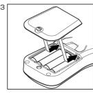
4. Screw the battery cover on the back of the instrument clockwise to lock the battery cover.
