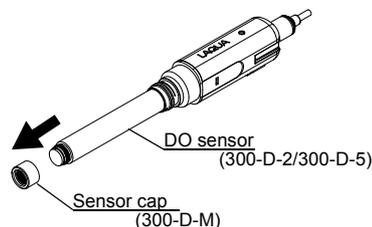
2. Tighten the new sensor cap on the DO sensor.
