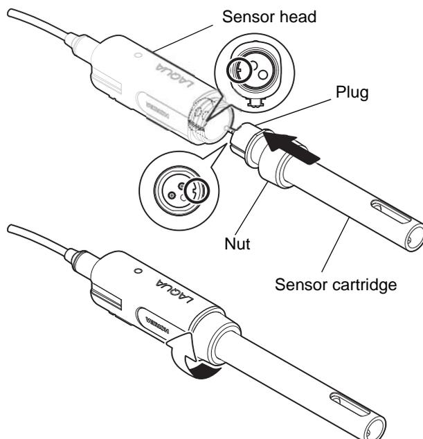
1. Connect the slot of the sensor cartridge with the marker of the sensor head and push into the sensor head.
