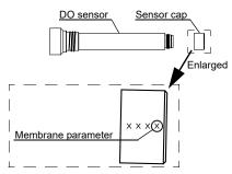
Perform "CAL in cap replacement" with the meter. The instruction procedure has been completed.
