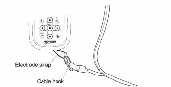
Note▶▶► Be sure to attach the cable hook to the electrode strap. If not, the cable may break.
