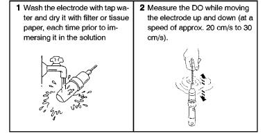
Note>>> The electrode membrane is thin and easily torn. Place it into solution slowly.
