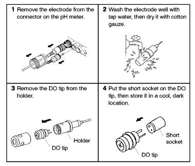
Note>>> Avoid storing the electrode in hot place or places with high humidity. Store the electrode indoors, out of direct sunlight.
