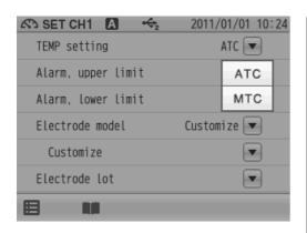
There are two types of temperature setting for ORP measurement; Automatic Temperature setting (ATC) and Manual Temperature setting (MTC).
