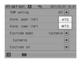
There are two types of temperature setting for mV measurement; Automatic Temperature setting (ATC) and Manual Temperature setting (MTC). In ATC, the instrument detects the solution temperature with the connected temperature sensor, and displays it on the screen. In MTC, measure the solution temperature and enter the value in advance. The instrument displays the entered temperature.
