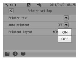
When a printer is connected with the instrument, this item allows you to perform an automatic printer test after measurement or calibration completion.
