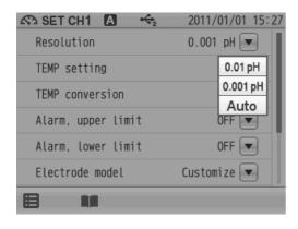
You can switch the resolution for pH measurement values to 0.01 pH, 0.001 pH, or Auto.
