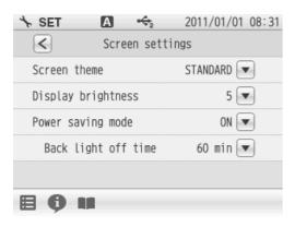
When selecting ON for Power saving mode, the Back light off time item is displayed.
