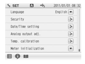
You can reset the instrument to the factory default conditions.
