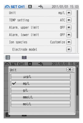
You can select  $\mu$ g/L, mg/L, g/L, mmol/L or mol/L as the ION measurement unit.
