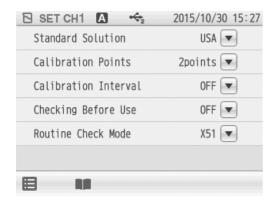
Up to 5 points calibration is possible. Set the number of the calibration points.
