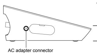
Insert the AC adapter cable by fitting with the connector socket of in the instrument.
