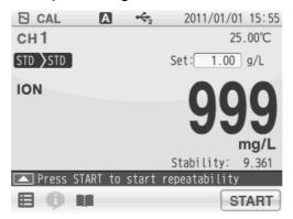
After the set point calibrations are completed, repeatability is automatically checked using the deviation between the calibrated and measured values at the 1st point.
