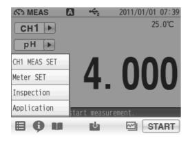
In the known addition method (Single), the targeted ion concentration in a sample solution is obtained from a change in electric potential by adding once a small amount of the target ion solution to the sample solution.
