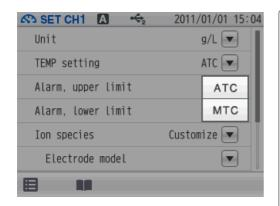
There are two types of temperature compensation for ION measurement; Automatic Temperature Compensation (ATC) and Manual Temperature Compensation (MTC). In ATC, the instrument detects the solution temperature with the connected temperature sensor, and performs temperature
