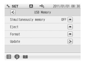
When a USB memory is inserted into the instrument, the data can be written into both the instrument and USB memories at the same time.
