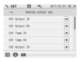
Connect the instrument with a digital multimeter, digital recorder, pen recorder or the like using a designated cable (analog output cable: Parts No.3014030152), and check and adjust the analog output value of the instrument.
