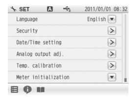
Security setting allows you to set a password for an administrator of the instrument.
