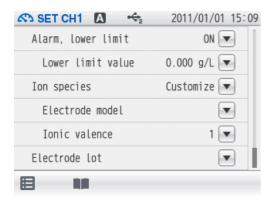
When an electrode lot No. is entered, the lot No. can be displayed on data printouts or recorded in saved data.
