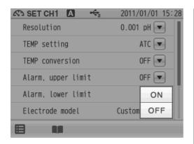
To use the temperature conversion function, set TEMP conversion to ON.
