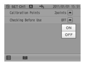
If you set the Checking Before Use setting to ON, it allows you to check repeatability after calibration by comparing the measured value of first point calibration standard solution with the calibration result.
