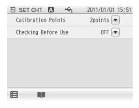
Up to 5 points calibration is possible. Set the number of the calibration points.
