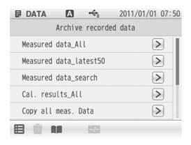
You can save the copy of the measurement data saved in the instrument into a USB memory. To execute the copy, connect a USB memory to the instrument.
