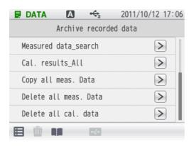
You can delete all measurement data saved in the instrument.
