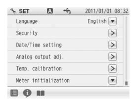
You can reset the instrument to the factory default conditions.
