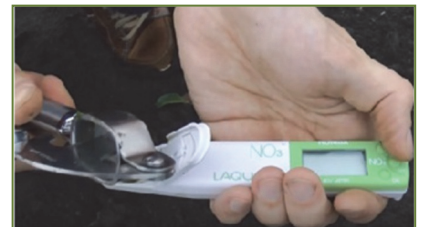
3. Pour the sap on the meter and measure.
