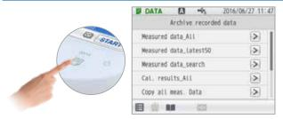
Data key shows settings that allow users to search, view, delete, and copy data from meter to USB flash drive
