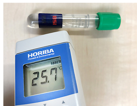
Figure 3. Horiba Infrared thermometer and blood collection tube for iCa measurement
