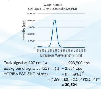
Note that this particular result exceeds the HORIBA minimum water Raman FSD specification for the QM-8075-11 spectrofluorometer when it is fitted with an optional cooled R928 PMT, which is currently specified at > 30,000:1 (FSD Method).
