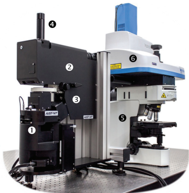
Figure 2 – Bolting the SPM and the spectrometer to an optical table forms a stable foundation. (1) SmartSPM with probe holder and sample stage; (2) OmegaScope with (3) two objective scanners; (4) video microscope for SPM navigation; (5) XploRA: full research confocal microscope; and (6) compact, powerful microspectrophotometer for conventional Raman and nano-Raman (TERS).
