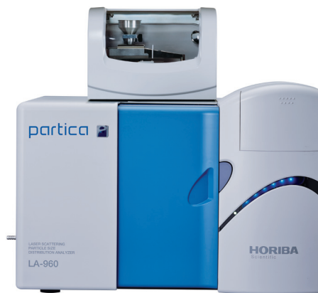
LA-960 Partica with PowderJet Feeder
