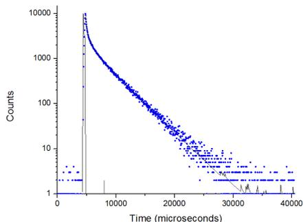
Figure 3: PL upconversion decay of Er<sup>3+</sup>-doped fluoride glass excited with 980 nm laser operating in the pulsed mode measured with MCS electronics. The decay is 3-exponential with lifetimes 213.3 (74%), 1000.3 (12.5%) and 3412 μs (13.5%). MCS acquisition was set for a total of 10,000 counts per peak channel and the decay acquisition time for these samples was 25 minutes (compared to 30 seconds for the SSTD data collected in figure 2).
