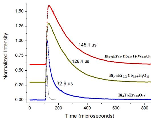
Figure 2: PL upconversion decays of three  $\text{Er}^{3+}$ -containing powders with varying composition of Yb and W excited with 980 nm laser operating in the pulsed mode. The decays were measured at the 546 nm emission peak. The total number of laser pulses was 10,000 and the total decay acquisition time for these samples was 30 seconds.
