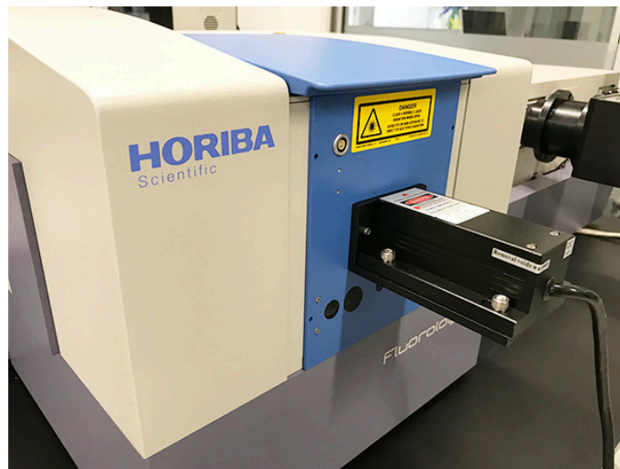
980 nm DPSS laser mounted to the front of the Fluorolog-QM sample compartment.
