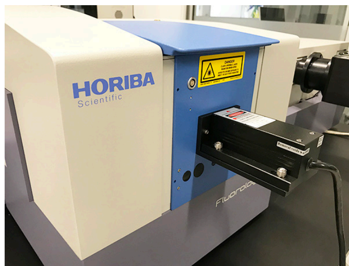
980 nm DPSS laser mounted to the front of the Fluorolog-QM sample compartment.
