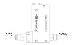
Gas inlet and outlet of the MFC fittings are 1/2inch VCR or equivalent with male screw fitting as standard. These MFCs can be mounted in any orientation, in most applications, without degradation of performance. Please make sure that process connections are as leak tight as possible.
