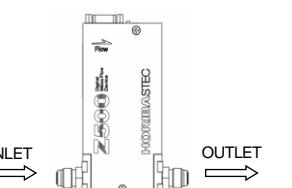
Gas inlet and outlet of the MFC fittings are 1/4inch VCR or equivalent with male screw fitting as standard. These MFCs can be mounted in any orientation, in most applications, without degradation of performance. Please make sure that process connections are as leak tight as possible. Confirm leak integrity of the installed MFC at the gas system connections using a helium mass spectrometer leak detector with sufficient sensitivity.
