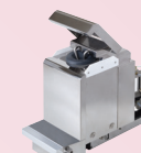
Mini flow with ultrasonic unit (0.01- 1000 \mu m)
