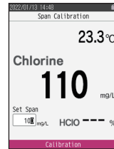
Span calibration screen
