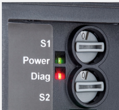
LED indicates status of diagnostics contact
