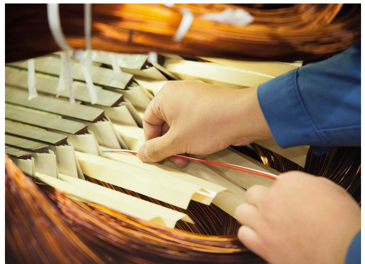
Image 4: Installation of a slot thermometer in an electric motor
