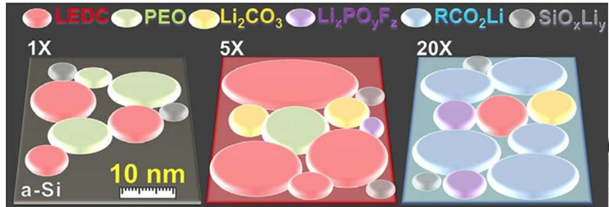
Figure1: Mosaic structure of various chemical compositions in the SEI layer after first, fifth and twentieth charge/discharge cycles. Clear evolution of chemistry and size of heterogeneities was demonstrated.
