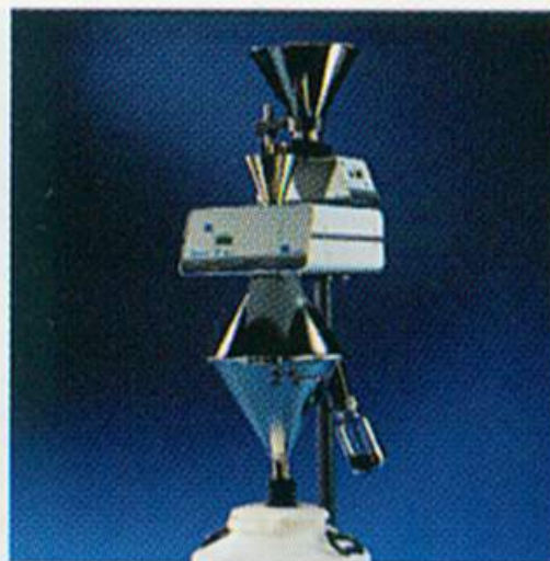
Laboratory rotary tube sample divider PKZ 1000
