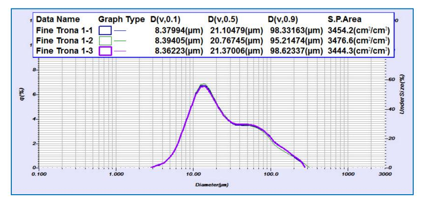
Measure particle size to screen incoming material and monitor milling end point, efficiency, etc.
