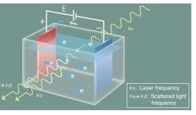
$\zeta$ :Zeta potential U:Electrical mobility E:Electric field strength n:Solvent refraction index  $\varepsilon$ :Solvent dielectric constant  $\eta$ :Solvent viscosity f( $\kappa a$ ):Henry coefficient
