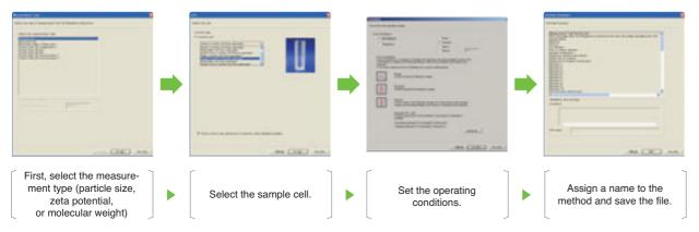
The software follows a progression of selecting measurement conditions and procedures and creates a navigation file.
