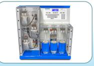
The Partica LA-960V2 is a laser diffraction particle size distribution analyzer that is known for its wide dynamic range, speed, excellent performance assurance, and outstanding quality. Its method expert software makes it easy to create a robust, powerful method for research and development purposes as well as quality control. The flexible sample handling, robust platform, and wide size range ensure the LA-960V2 will handle the most extreme demands.
