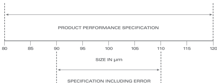
figure 16 BUILDING SIZE SPECIFICATION TO INCLUDE ERROR SOURCES If the total measurement error is +/- 10%, then the specification must be tightened in order to assure the product stays within performance specification.
