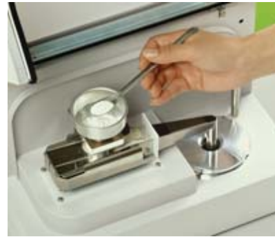
Figure 2: Dry Powder Feeder
