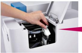
The flow cell cleaning is one of the most essential maintenance routine. Therefore it should be easily handled by anyone who operates the analyzer. The system is designed to keep enough space in the cell chamber for easy operations.
