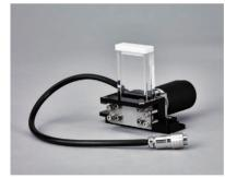
The Fraction cell optional accessory enables measurement of very limited sample amounts and collecting them after the measurement. The stir bar inside of the cell prevents the particle segregation and sedimentation.
