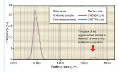
Comparison of the results of undiluted suspension measurement and flow measurement (diluted with dispersant)
