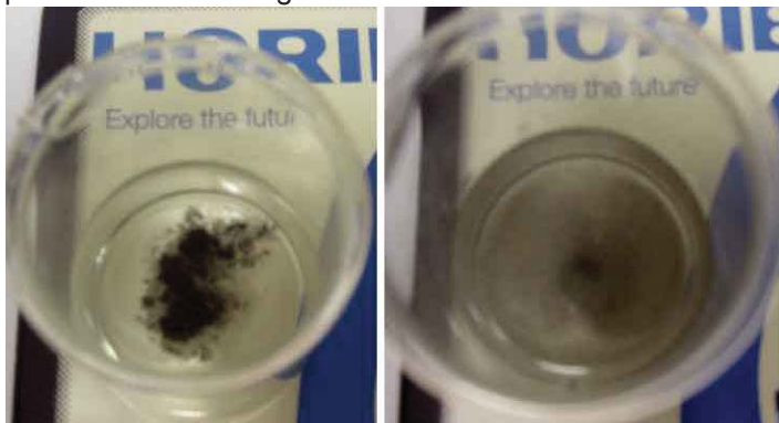
Figure 2: Left; non-wetted powder, Right; wetted after surfactant is added
