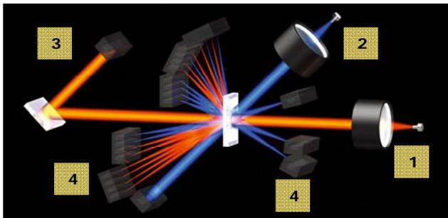
Figure 4: A simplified layout of the LA-950 optical bench. 1: Red wavelength laser diode for particles > 500 nm, 2: Blue LED for particles < 500 nm, 3: Low angle detectors for large particles, 4: Side and back angle detectors for smaller particles.
