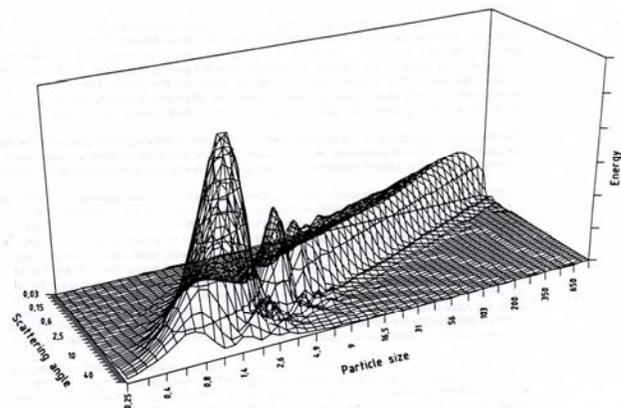
Light energy scattering patterns for an arbitrary detector configuration against particle size (μm) and scattering angle (°) for equal volumes of particles (Mie theory, latex particles RI 1.60 - 0.0i, in water RI 1.33)
