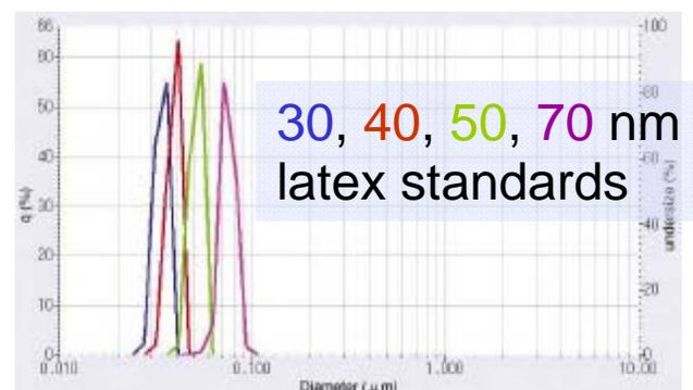
Figure 7: 30, 40, 50, and 70 nanometer materials independently measured on the LA-950 using the blue LED
