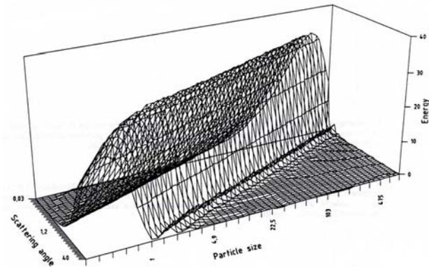
Light energy scattering patterns for an arbitrary detector configuration against particle size (μm) and scattering angle (°) for equal volumes of particles (Fraunhofer theory)
