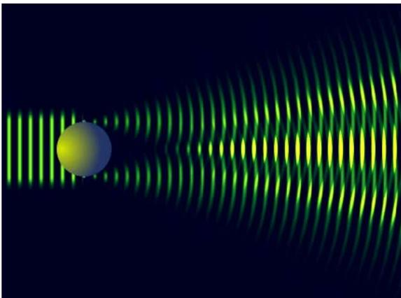
Figure 1: The diffraction pattern (right side) of a plane wave scattering off a spheroid (left side).
