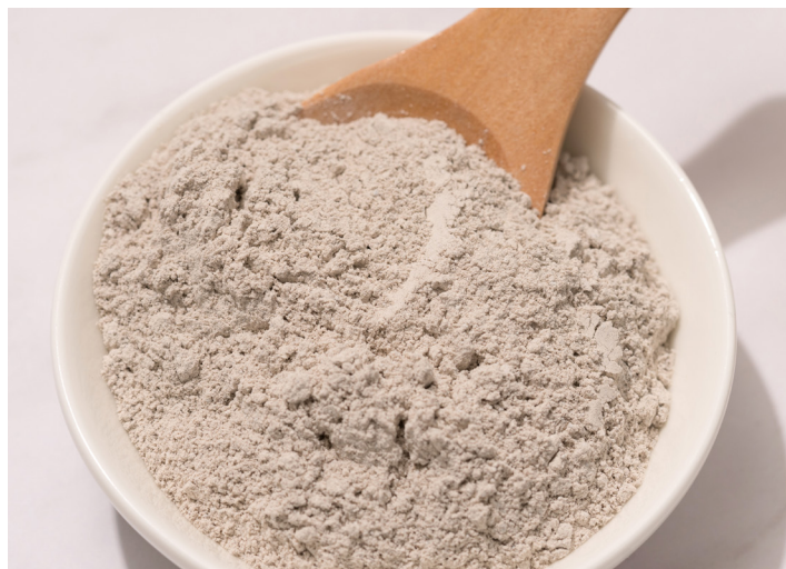
Figure 1. Example of bentonite powder.
