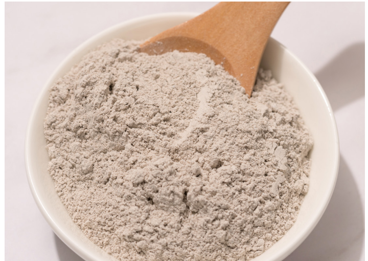
Figure 1. Example of bentonite powder.
