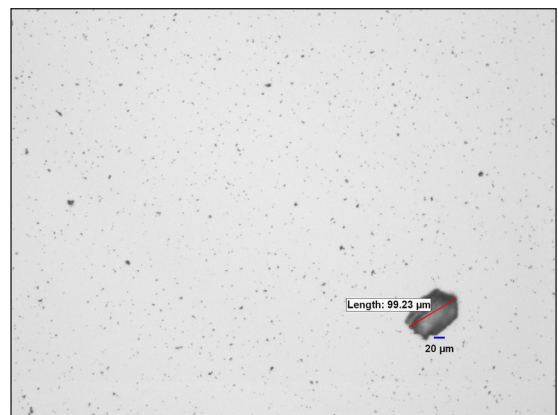
Figure 6: Large Particle 1 from DPI
