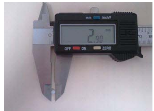
Figure 1: Size of a plastic bead measured by caliper
