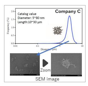
As a result of measuring CNTs made by Company C, only the particle size distribution that seems to be derived from aggregated CNTs was obtained, and SEM observation showed that there were almost no isolated CNTs, but only aggregated CNTs. The particle size distribution shows the state of the CNTs.
