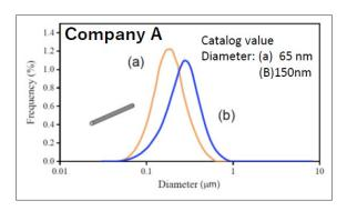
Both types of CNTs made by Company A were found to be isolated and dispersed and the CNTs with different diameters had different particle size distributions. The measured particle size also depends on the length of the CNTs, which indicates that the difference in diameter of the isolated CNTs can be analyzed.
