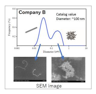
The measurement of CNTs made by Company B resulted in a two peak particle size distribution. A and SEM observation showed both isolated and aggregated CNTs. It suggests that the particle size distribution represented each component.
