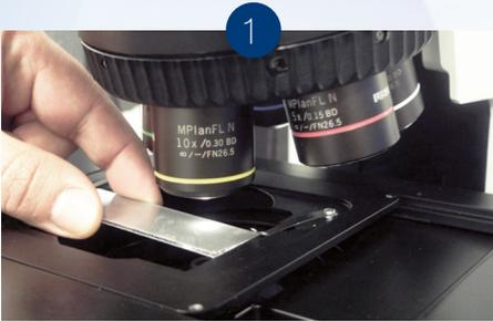
Place the patterned substrate in the field of view of camera or microscope
