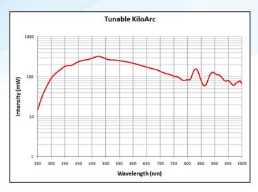
Tunable KiloArc<sup>TM</sup> Illuminator equipped with 1000 watt Xenon lamp and 1,200  $I/mm \times 500$  nm blazed grating. Here the adjustable bandpass was set to 20 nm.
