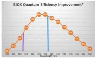
Synapse EM-BIQX provides enhanced QE for UV Raman laser line \*Compared to conventional back-illuminated sensor
