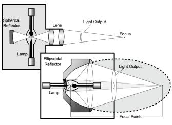
For the same bulb, the PowerArc<sup>™</sup> delivers 5 to 6 times more light to the secondary focus! That means that an PowerArc<sup>™</sup> lamp housing with a 75 watt xenon lamp provides the equivalent optical power of a 450 watt xenon lamp in an old style vertical lamp housing. And it does so with greater power density due to a smaller focal spot, and at a small fraction of the cost of a big old 450 watt illuminator.
