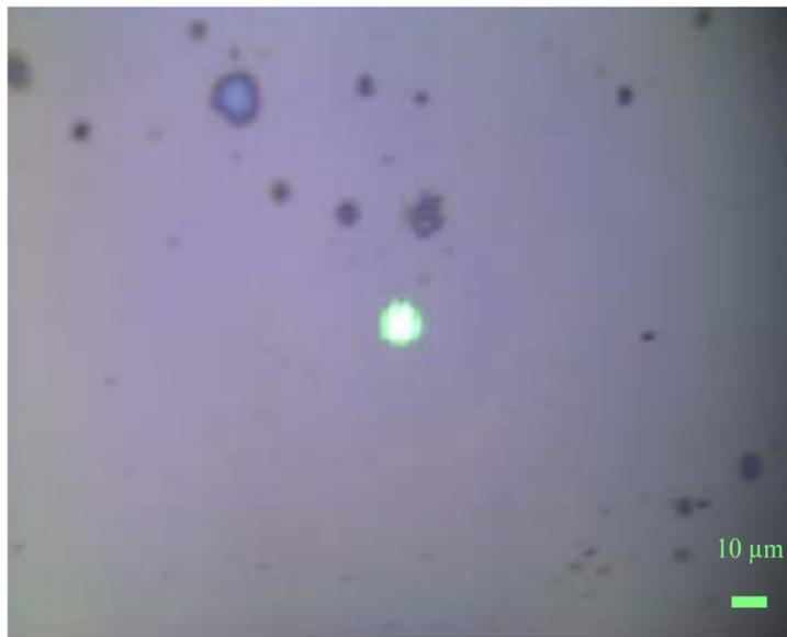
Figure 5: Tightly focused excitation laser spot on the sample. This spot excitation is scanned across a region of interest in a raster fashion to generate a 2D map.
