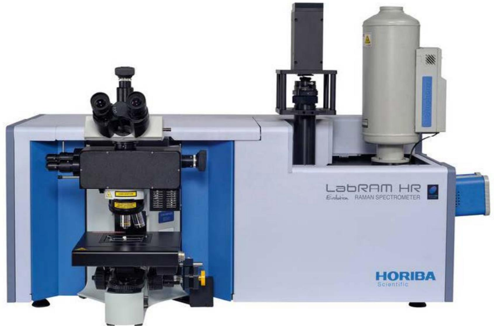
LabRAM HR Evolution Confocal Raman/PL microscope
