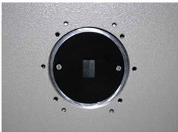
FHR after removal of four mounting screws
