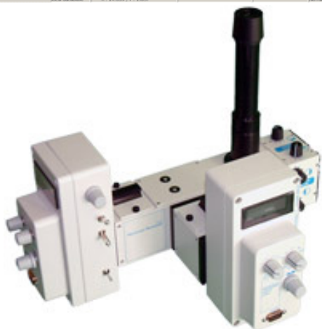
Dual emission channel HORIBA photometer for Indo-1 Ca 2+ measurements
