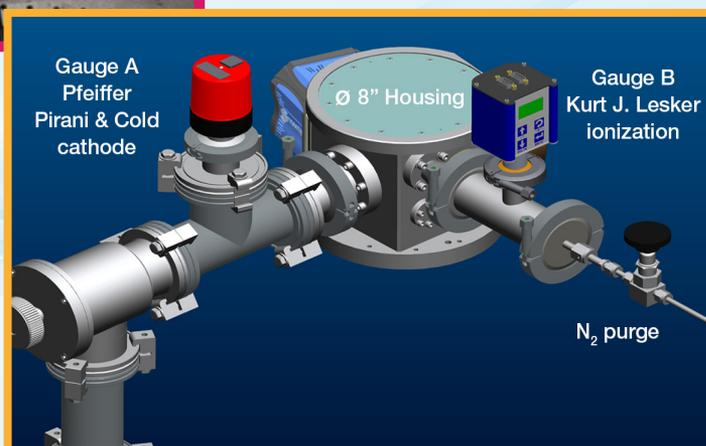
$\text{N}_2$ -purged set-up shown with Hamamatsu: L10366 VUV light source
