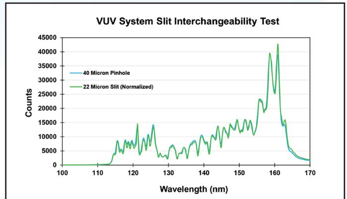
VUV system slit interchangeability test with 40 μm pinhole and 22 μm slit
