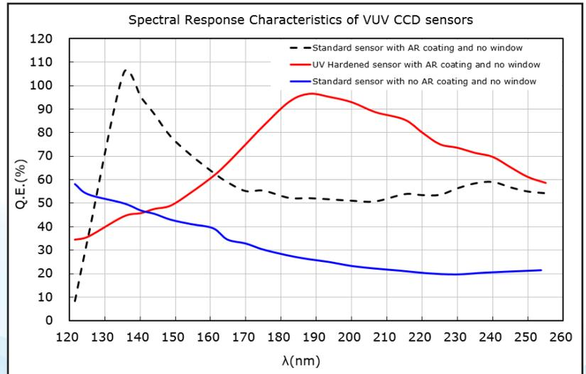
UV hardened sensor provides increased lifetime, however no warranty is provided on any sensor exposed to VUV.
