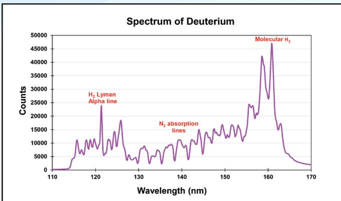
Spectrum of deuterium lamp shows enhanced sensitivity starting from 113 nm with 22 μm slit (0.45 nm resolution)
