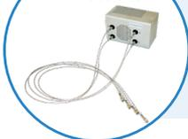
CCD spectrometer for simultaneous acquisition from 4 fiber inputs (470-730 nm)
