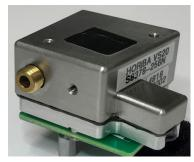
Spectrometer housing for S8378 sensor
