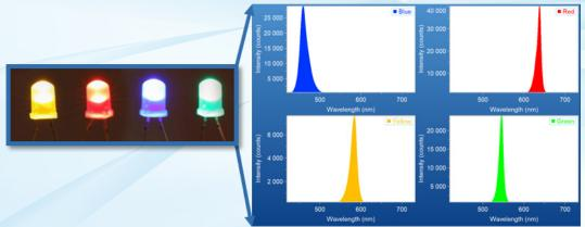
PoliSpectra Quad Spectrometer is capable of simultaneously measuring 4 channels of 1024 pixels spectra. The picture above shows the emission spectra of 4 different color LEDs measured using  $\emptyset$  200 µm core fibers.
